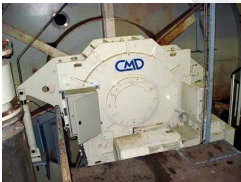
Jumboflex® worm gearbox for sugar beet crystalliser
