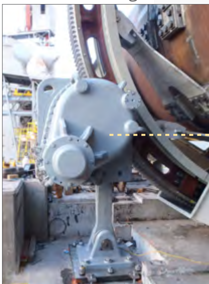
Bogiflex ® KGD self-aligning kiln gear drive
